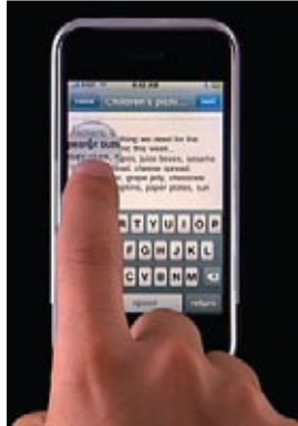
Figure 2-22. The iPhone provides a drag magnifier lens that makes it easier to position the cursor
