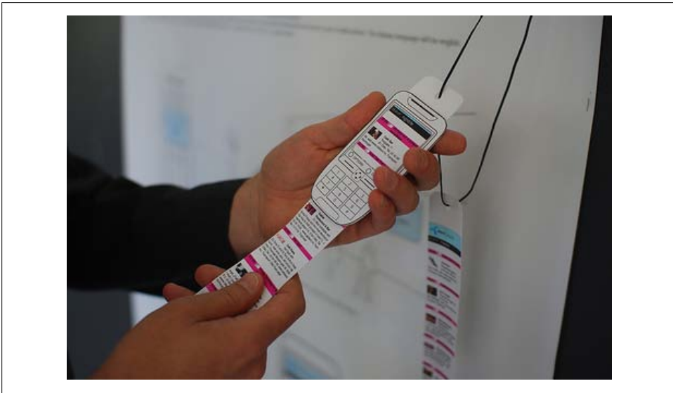
Figure 7-11. A paper prototype, where the interaction is nothing more than drawings on note cards
