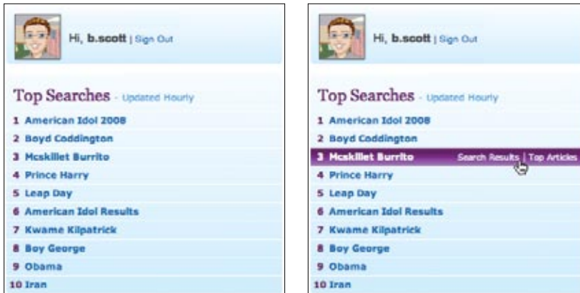
Figure 4-10. Yahoo! Buzz reveals additional tools for the top searches when the user hovers over each item
